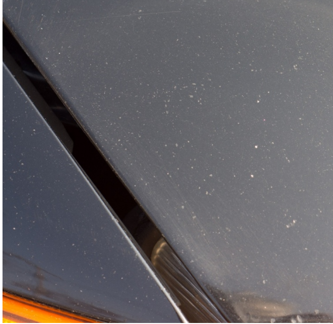
Photo 3: In this photo you can see the longevity of a 1K UV-A primer and a 1K UV-A Clear Coat after 8 years of service in the Northeastern US.
