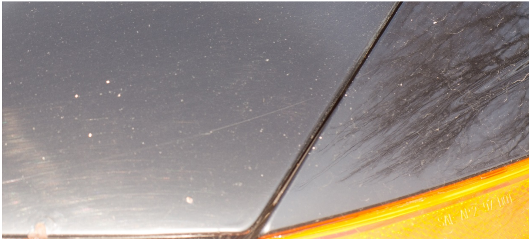
Photo 4: In this photo you can see the longevity of a 2K PUR primer and Clear Coat as the standard for comparing against the 1K UV-A primer and a 1K UV-A clear coat after 8 years of service in the Northeastern US.
